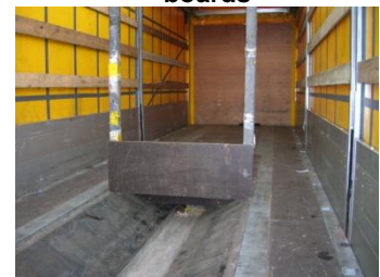
Clean and tidy coil well
