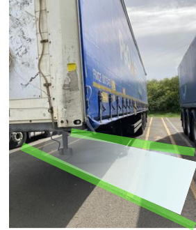
Park trailer legs on concrete strip
