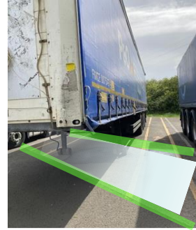
Park trailer legs on concrete strip
