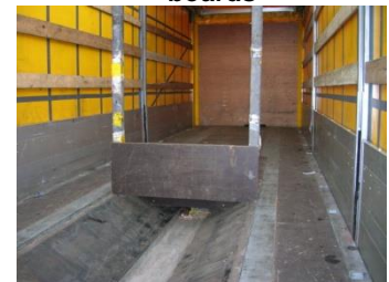
Clean and tidy coil well
