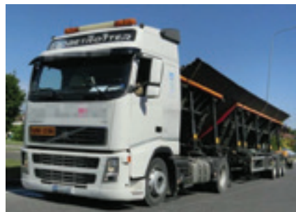
Figure 14: Steel plates transported under 45°
