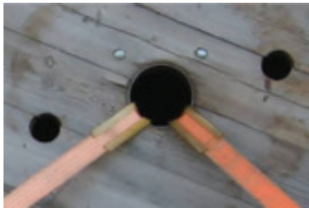
Figure 22: Protection at sharp edges
