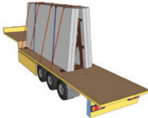
Figure 48: Securing with combination of blocking, A-frame, round lashing and top-over lashing
