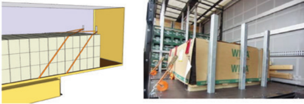
Figure 7: Stanchions used for blocking in forward direction
