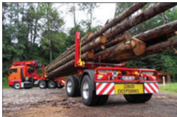
Figure 54: Securing of whole trees
