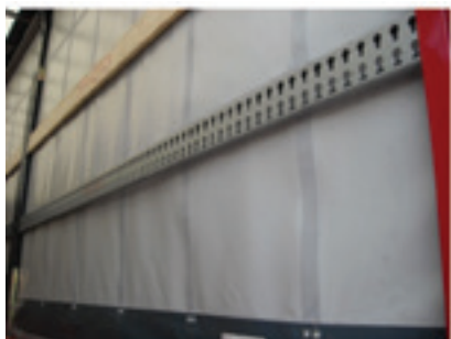
Figure 27: Alu lath with wholes for blocking bars
