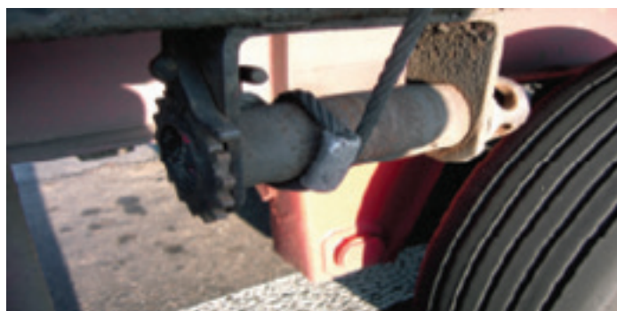
Figure 24: Steel wire rope tensioned by winch
