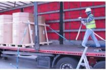
Driver positions wooden frame and puts cordstrap around the wood and places the friction mats.
