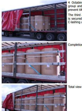
4 Octabins are arranged together in a group and are secured with cordstrap to prevent tilting.
