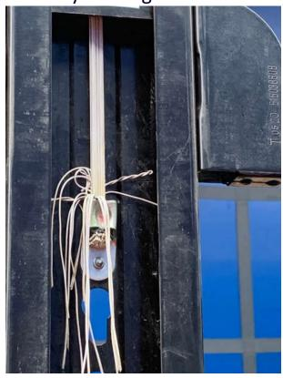
**Findings** – Internal Tension Cable severely overstretched. This type of roof support is common on different types of trailers not just Mega trailers.
