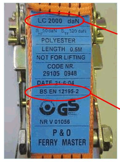
Lashing Capacity 2000 daN – This is 2ton of Force NOT Weight!
