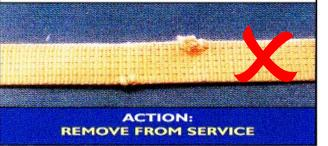
The webbing has been cut across its width by a sharp edge. This type of damage will result in substantial loss of strength.
