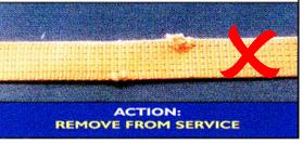
The webbing has been cut across its width by a sharp edge. This type of damage will result in substantial loss of strength. ACTION: **REMOVE FROM SERVICE** Knotted webbing should not be used. A cut lashing should not be joined by knotting.
