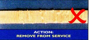
Knotted webbing should not be used. A cut lashing should not be joined by knotting.
