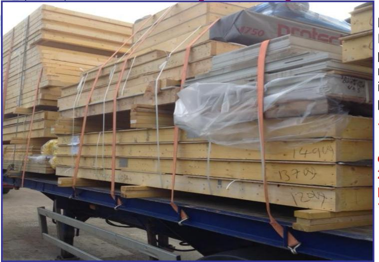
Mixed load of External wall panels, Loose material and internal wall panels **10m Straps.**
