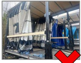
Trailer **MUST NOT** be left in this condition. **All** boards are to be removed
